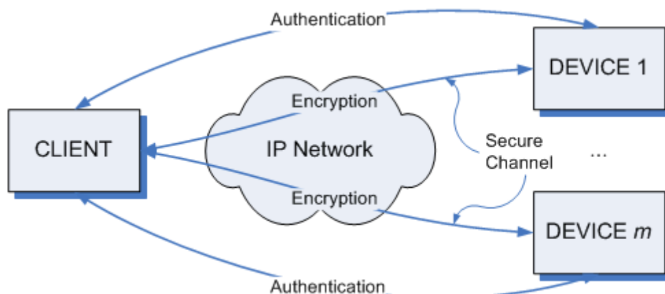
1019 1020 Figure 2: Communication mechanisms for authentication information and for encrypted messages 1021 The organization of CLIENT and DEVICE credentials, mechanism for provisioning them, and criteria for 1022 distinguishing valid and invalid credentials is out of scope of this profile.
