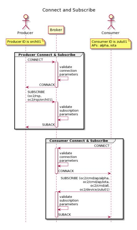
The Producer and Consumer CONNECT packets for this example are as follows; the optional username and password fields of the CONNECT packets are populated in this example:
