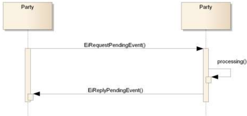
1750 1751 Figure 9-7: Interaction Diagram for Pending Event operation
