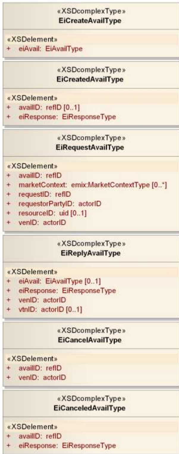
1880 1881 Figure 11-3: UML Class Diagram for EiAvail Service Operation Payloads
