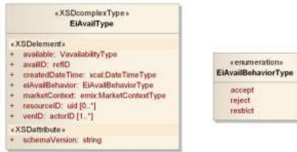
1876 Figure 11-2: UML Class Diagram for the EiAvail Type
