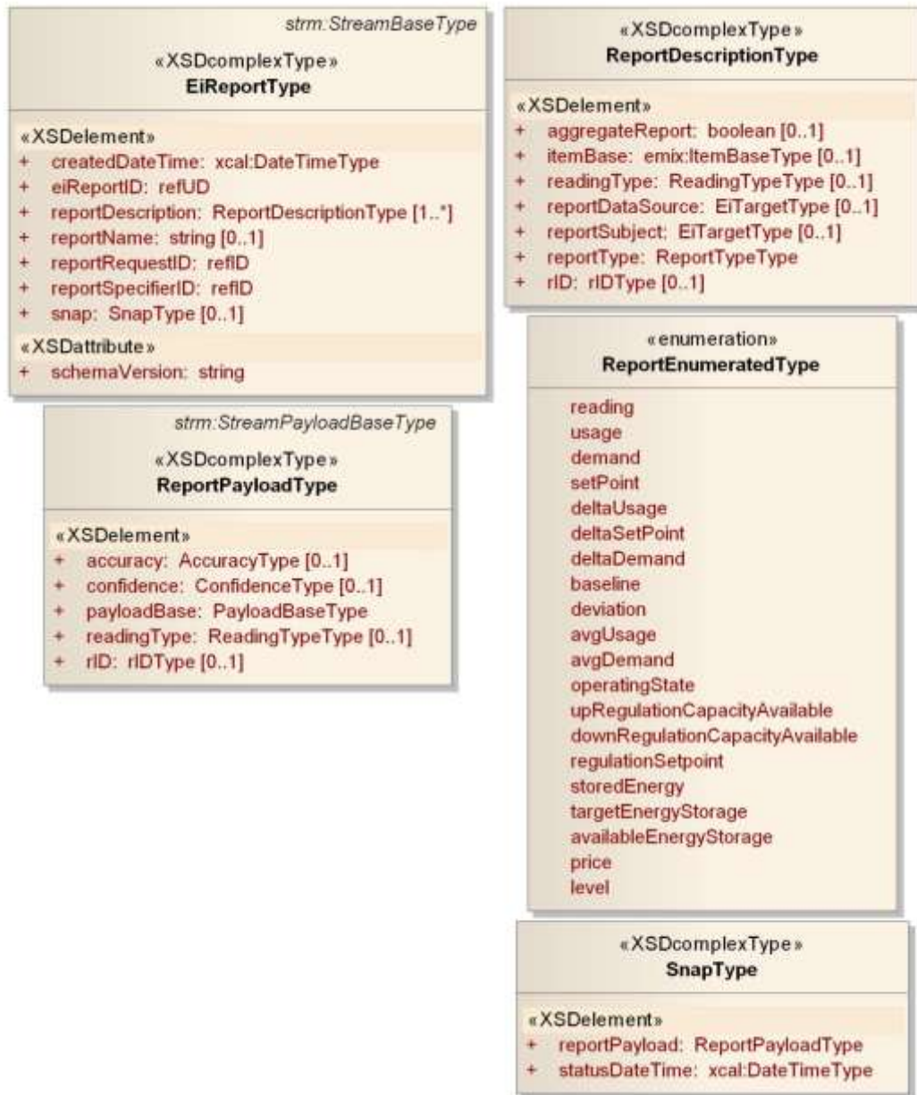
1263 1264 Figure 5-16: UML Class Diagram of Reports 1265
