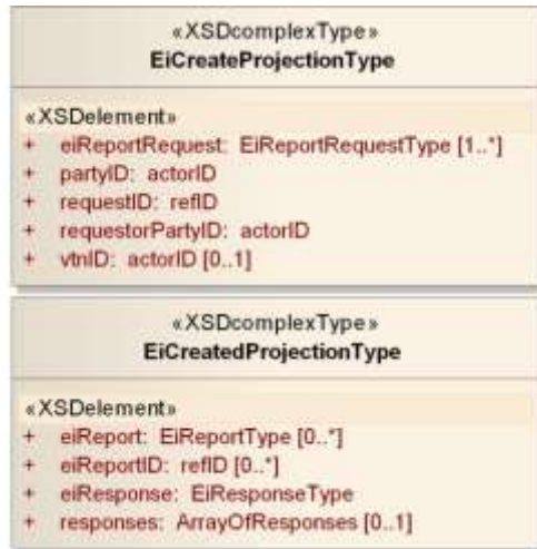
1813 1814 Figure 10-7: UML Diagram of Projection Payloads
