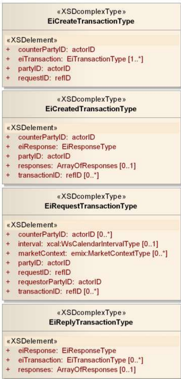
1586 Figure 7-9: UML Class Diagram of EiTransaction Service Operation Payloads
