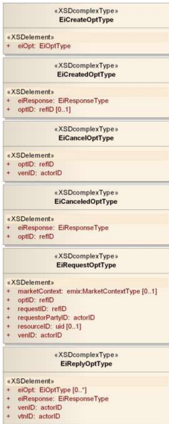
1904 1905 Figure 11-6: UML Class Diagram for EiOpt Service Operation Payloads
