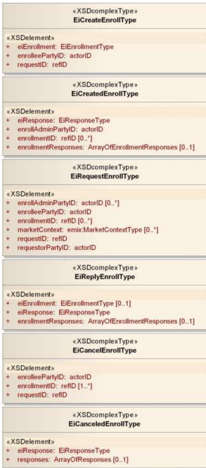
1658 Figure 8-4: UML Class Diagram for Enrollment Payloads
