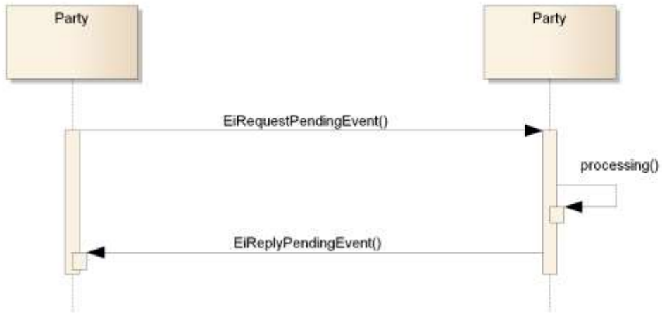
1763 Figure 9-7: Interaction Diagram for Pending Event operation
