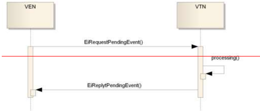
1757 1758 Figure 9-6: UML for example PULL pattern for EiEvent 1759 1760
