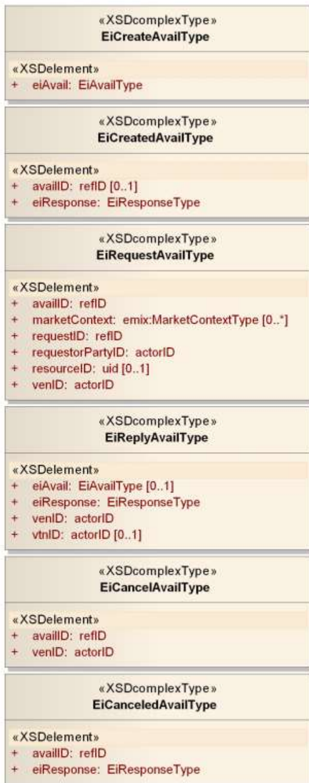
1913 Figure 11-3: UML Class Diagram for EiAvail Service Operation Payloads
