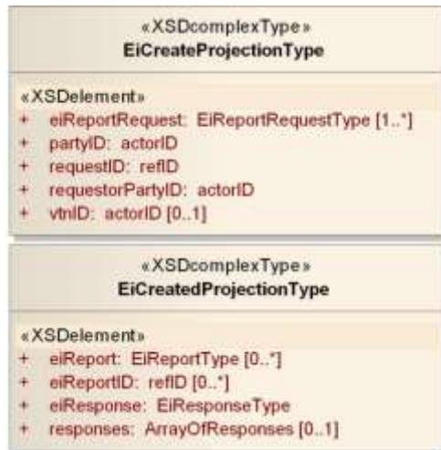
Figure 10-7: UML Diagram of Projection Payloads
