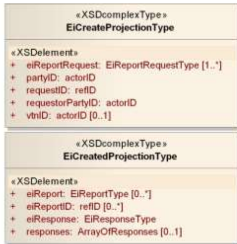
1821 Figure 10 : UML Diagram of Projection Payloads
