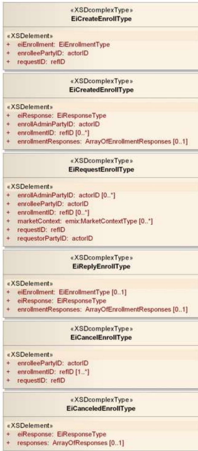
1669 Figure 8-4: UML Class Diagram for Enrollment Payloads
