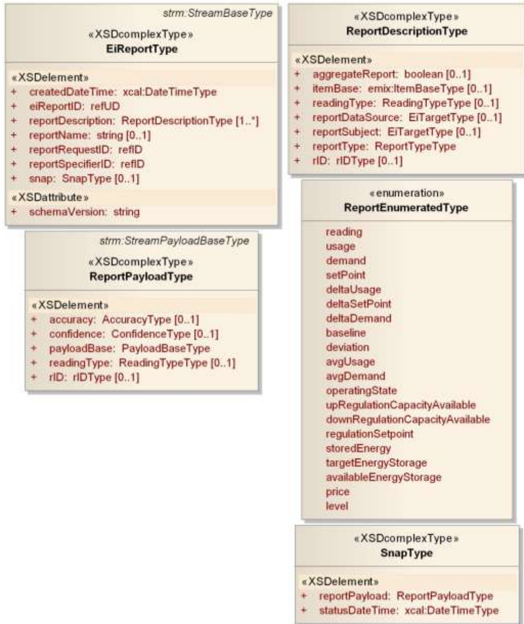
1269 1270 Figure 5-16: UML Class Diagram of Reports 1271
