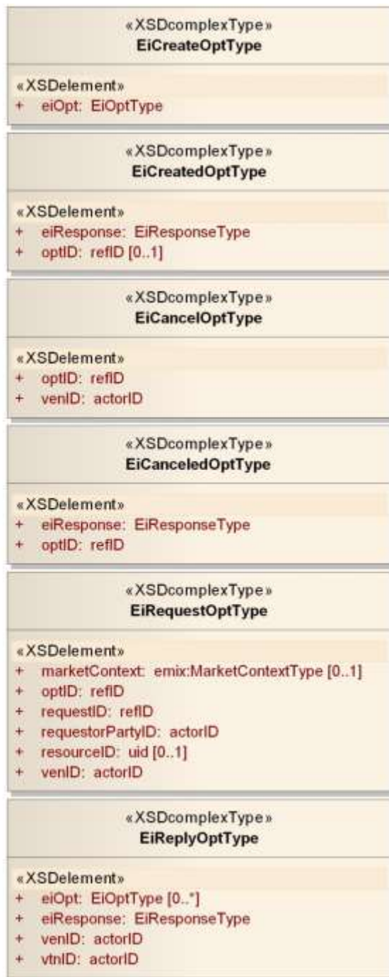
1937 Figure 11-6: UML Class Diagram for EiOpt Service Operation Payloads
