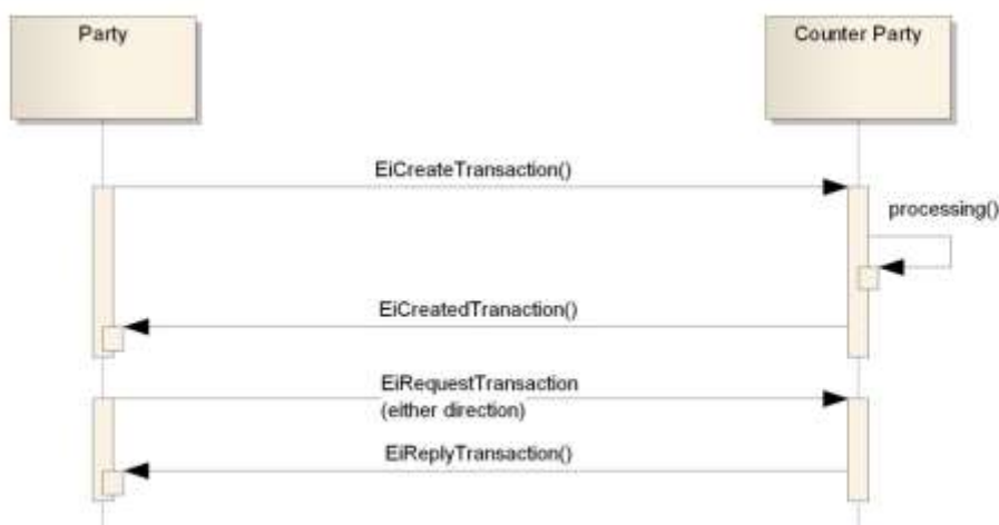
1587 | 1588 | Figure 7-8: Interaction Diagram for the EiTransaction Service
