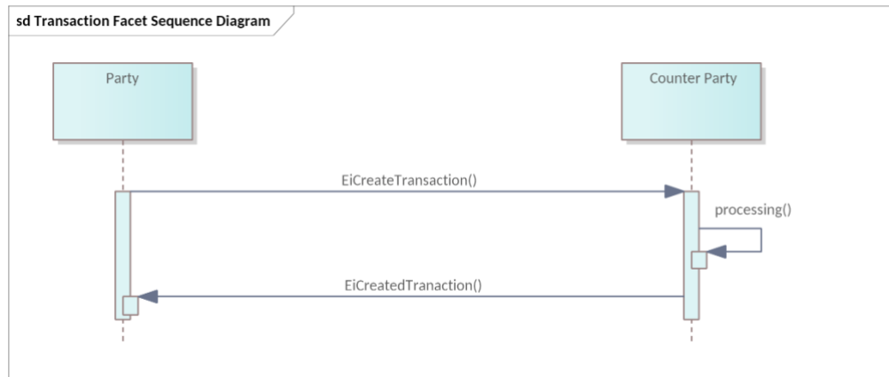
Figure 6-1: UML Sequence Diagram for the EiTransaction Facet
