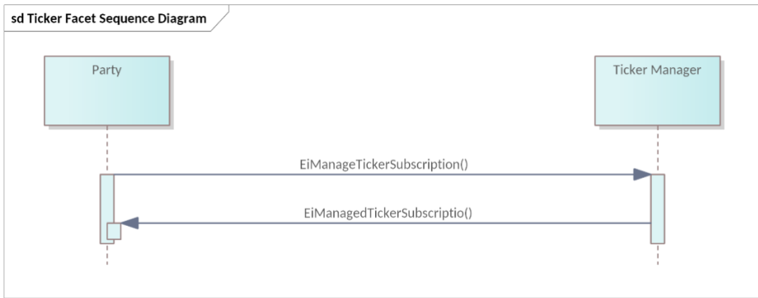
Figure 11-2: UML Sequence Diagram for the Ticker Facet
