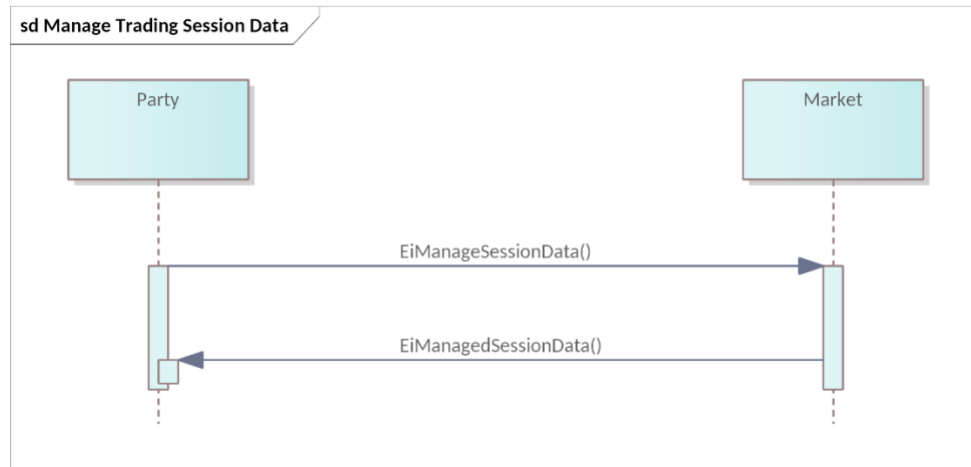
Figure 13-8: UML Sequence Diagram for Manage Trading Session Data
