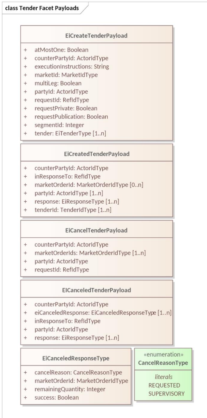
Figure 5-4 UML Class Diagram for Tender Facet Payloads
