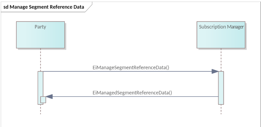
1899 1900 Figure 13-5 UML Sequence Diagram for Segment Reference Data
