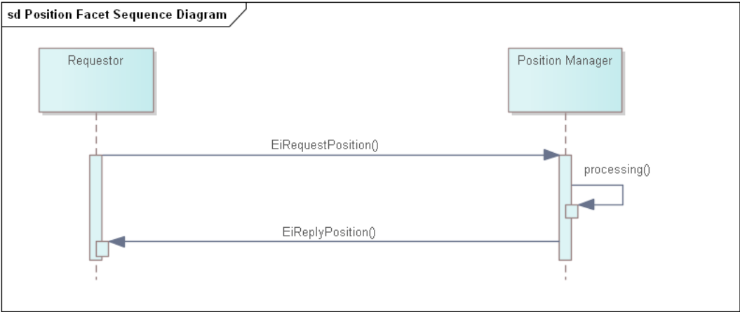
Figure 7-1: UML Sequence Diagram for the Position Facet
