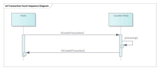
Figure 6-1: UML Sequence Diagram for the EiTransaction Facet
