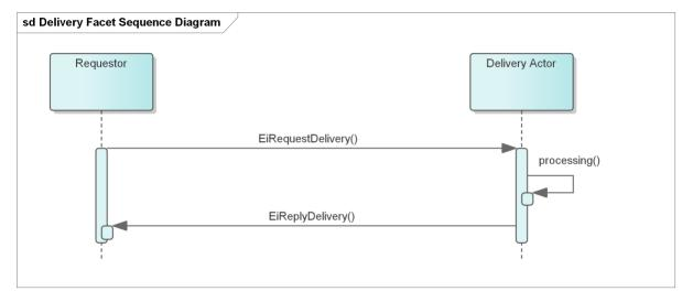
Figure 8-1: UML Sequence Diagram for the Delivery Facet
