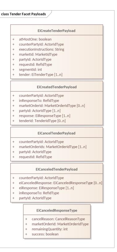
Figure 5-4 UML Class Diagram for Tender Facet Payloads
