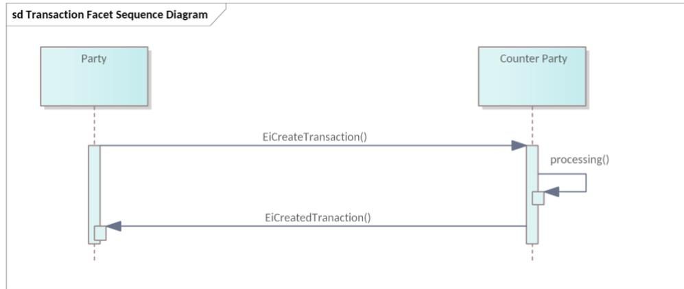
Figure 6-1: UML Sequence Diagram for the EiTransaction Facet
