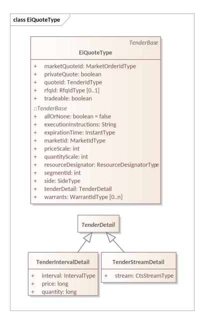
Figure 9-7 UML Class Diagram of EiQuoteType showing inherited attributes.
