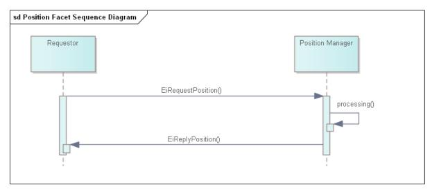
Figure 7-1: UML Sequence Diagram for the Position Facet
