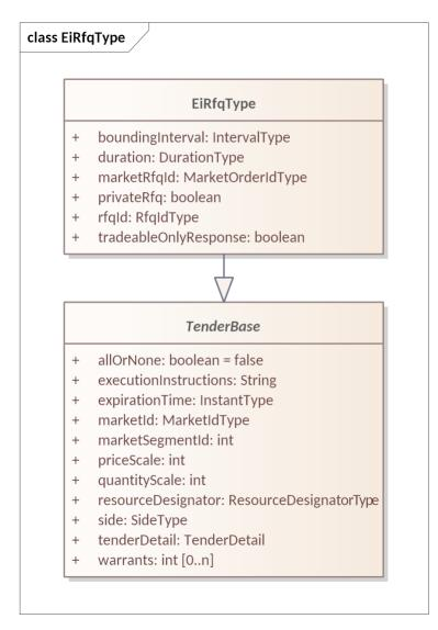
Figure 9-6 UML Class Diagram for EiRfqType
