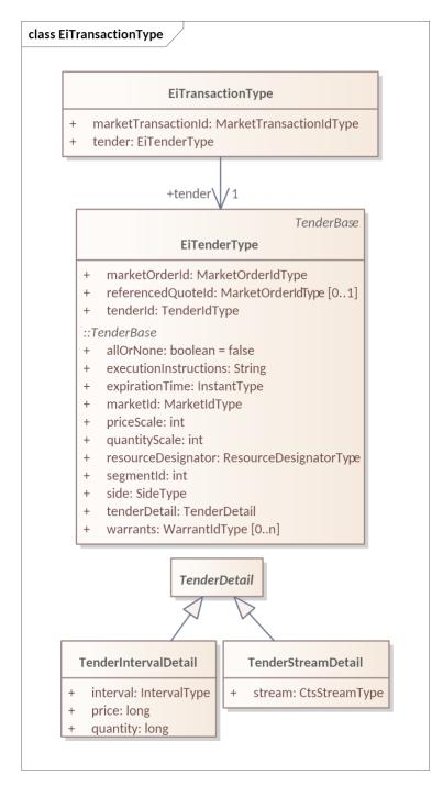
Figure 6-2: UML Class Diagram of EiTransactionType
