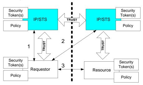
Figure 8: Federation and Trust Model
