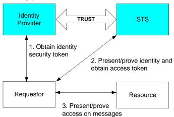
Figure 14: Role of IP/STS in Basic Federation Model
