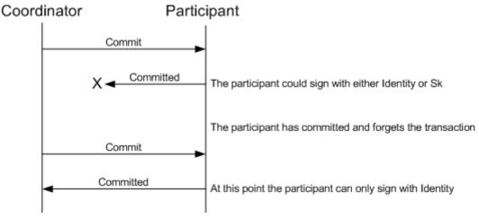
There are, of course, techniques to mitigate this situation but such options will not always be successful. Consequently, when dealing with Atomic Transactions, it is critical that identity claims always be proven to ensure that correct access control is maintained by coordinators.
