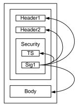
Note: if required, the initiator may also include in the Security header the token used as the basis for the message signature (Sig1), not shown in the diagram.
