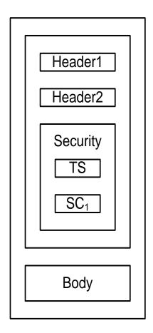
The outer box shows that the entire message is protected (signed and encrypted) by the transport. One wssell:SignatureConfirmation element labeled SC<sub>1</sub> corresponding to the signature in the initial message illustrated previously is included. In general, the ordering of the items in the security header follows the most optimal layout for a receiver to process its contents.
