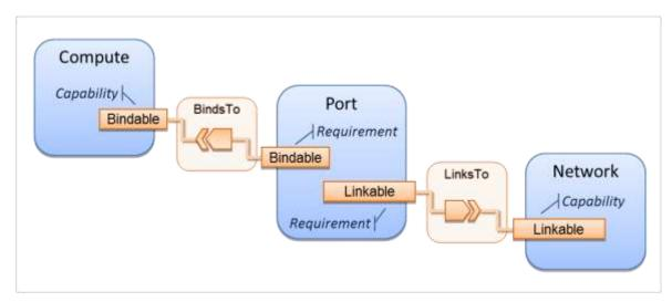
As you can see, the Port node type effectively acts a broker node between the Network node description and a host Compute node of an application.
