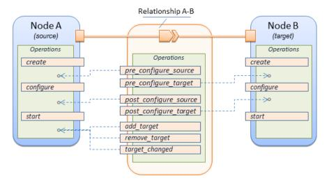
TOSCA relationships are directional connecting a source node to a target node. When TOSCA Orchestrator connects a source and target node together using a relationship that supports the Configure interface it will "interleave" the operations invocations of the Configure interface with those of the node's own Standard lifecycle interface. This concept is illustrated below:
