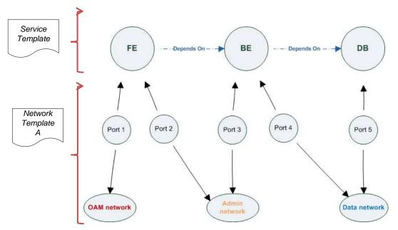
Figure-7: Service template with network template A
