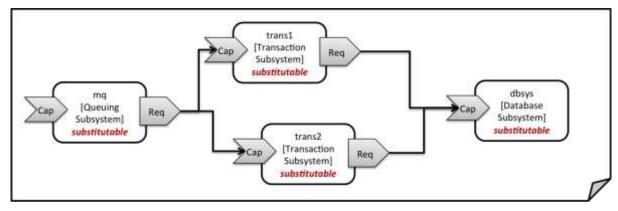
Figure 3: Chaining of subsystems in a service template
