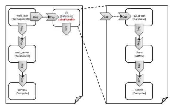
Figure 1: Using template substitution to implement a database tier
