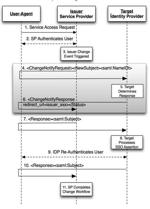
Figure 2: Change Notify Web SSO at Service Provider
