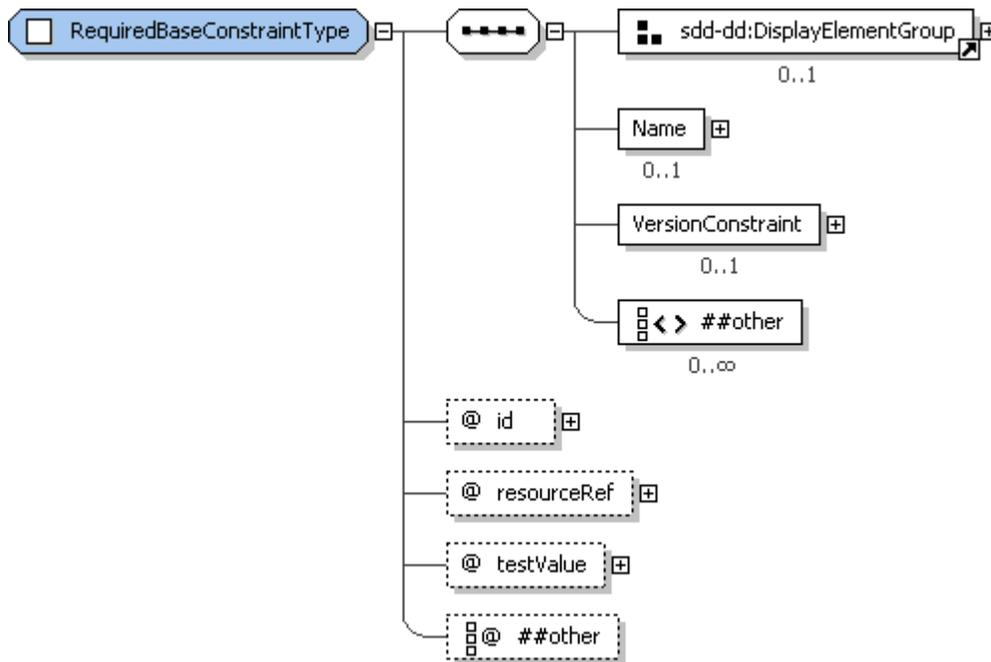
2599 **Figure 68: RequiredBaseConstraintType structure.**
