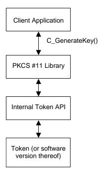
Figure 3: Generation of an OTP key
