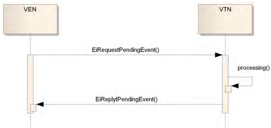
Figure 9-7: Interaction Diagram for Pending Event operation
