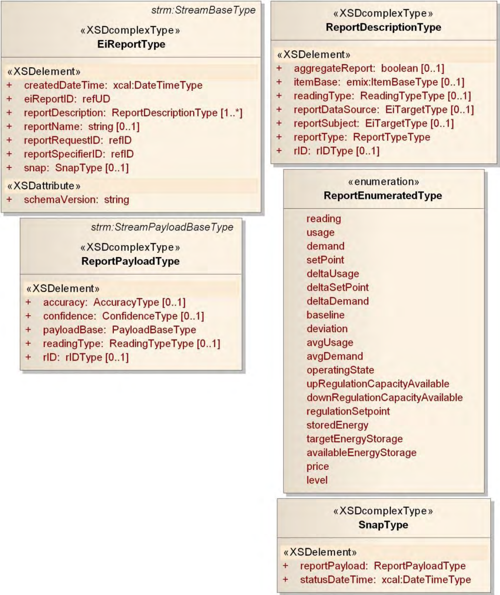
1246 1247 Figure 5-16: UML Class Diagram of Reports
