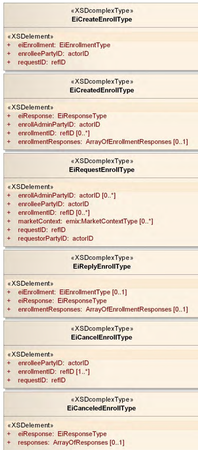
Figure 8-4: UML Class Diagram for Enrollment Payloads
