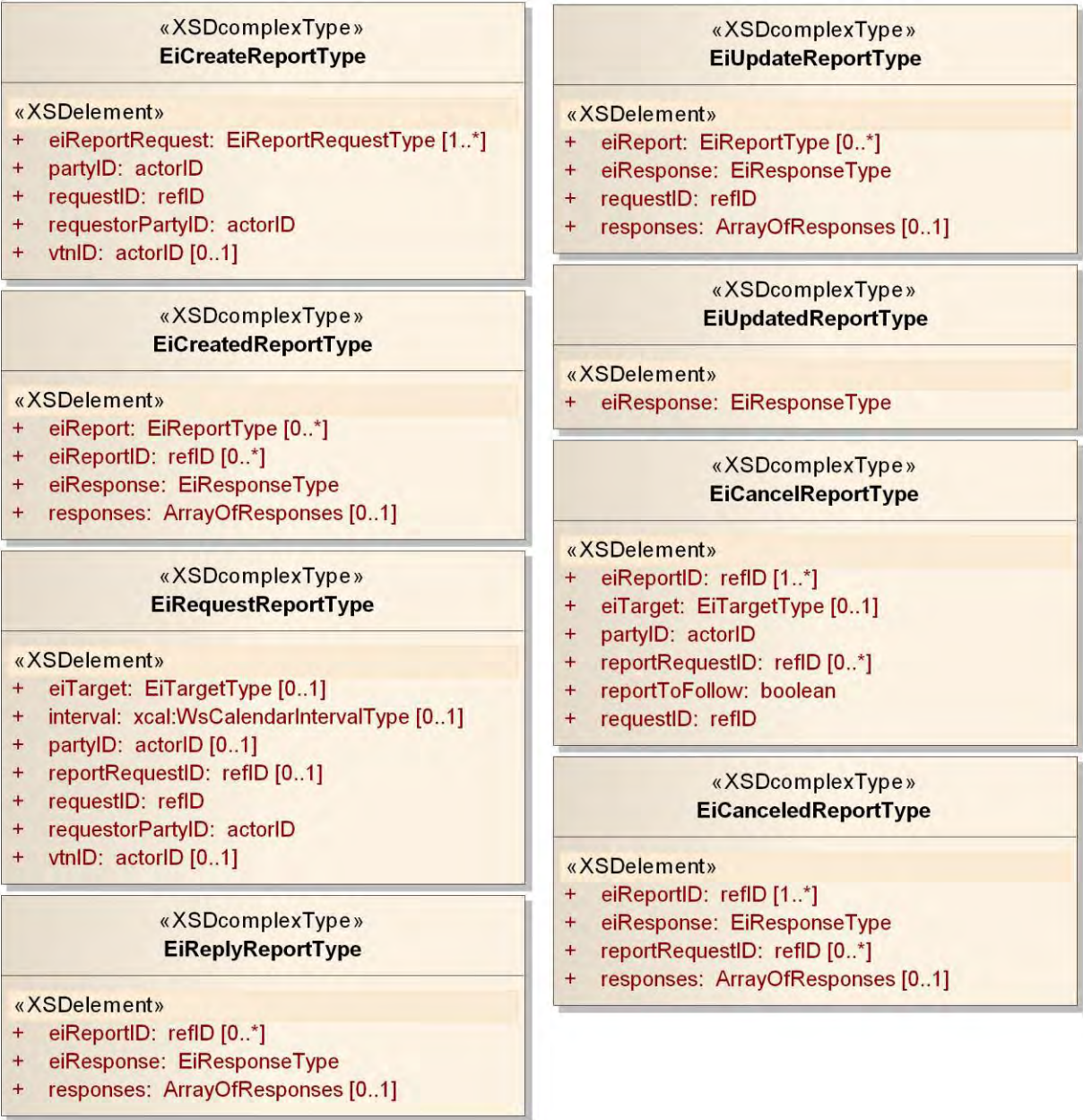
Figure 10-4: UML Diagram of Report Payloads
