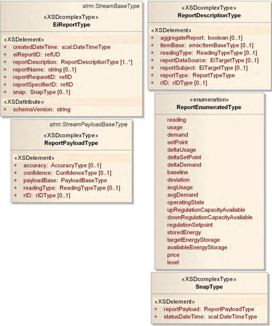
Figure 10-7: UML Class Diagram for the EiReport Class
