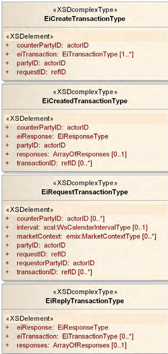
1567 1568 Figure 7-9: UML Class Diagram of EiTransaction Service Operation Payloads
