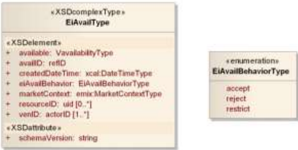
1889 1890 Figure 11-2: UML Class Diagram for the EiAvail Type 1891
