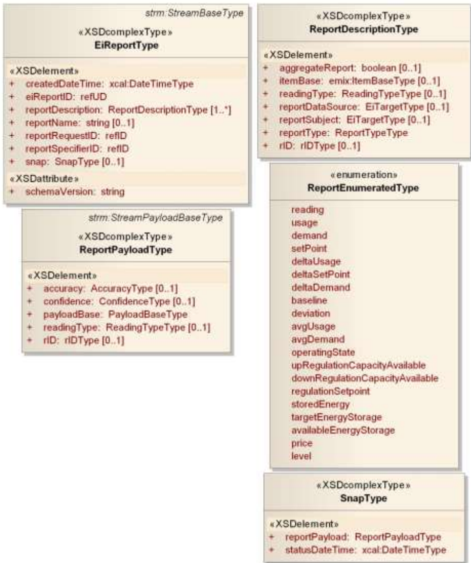
Figure 10-3: UML Class Diagram for the EiReport Class
