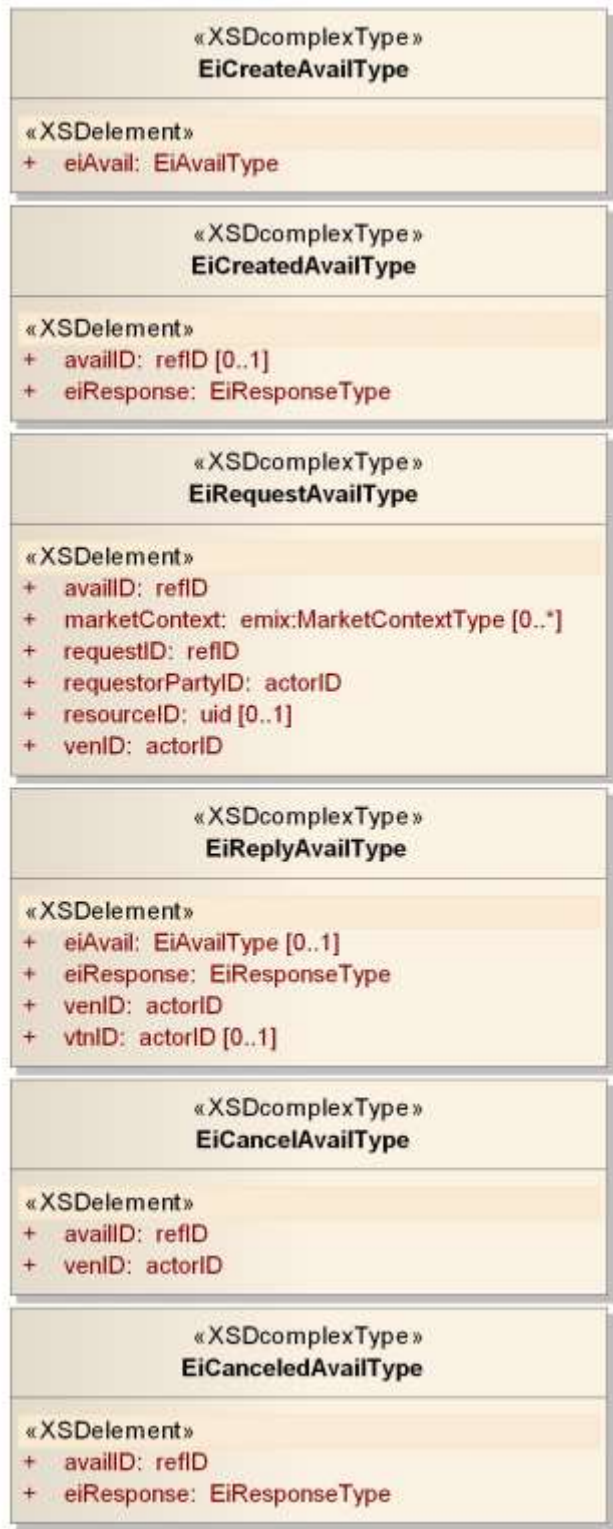
Figure 11-3: UML Class Diagram for EiAvail Service Operation Payloads
