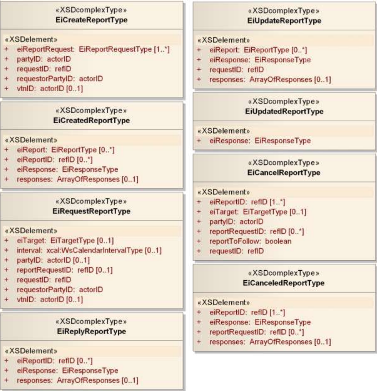
Figure 10-5: UML Diagram of Report Payloads
