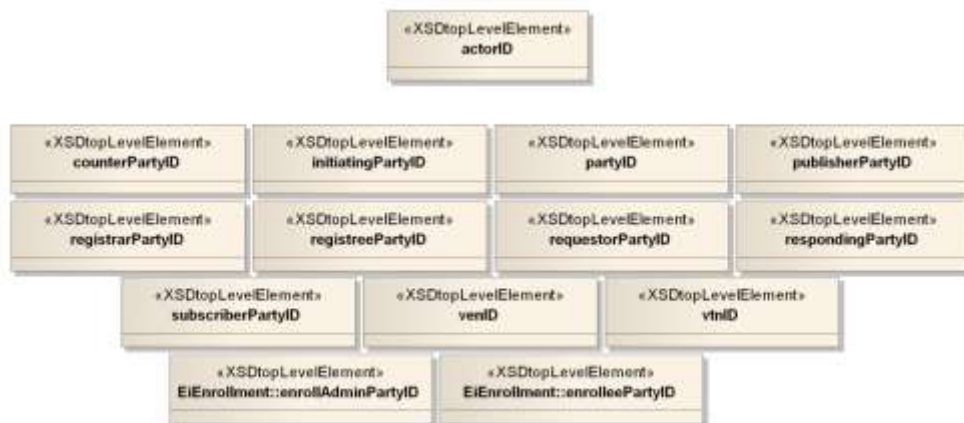
Figure 5-2: UML Class Diagram of Party ID and its derivatives
