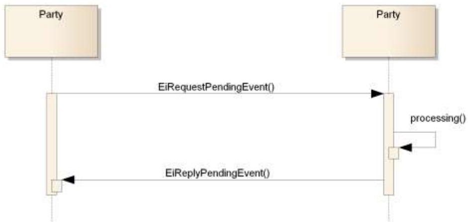
Figure 9-7: Interaction Diagram for Pending Event operation
