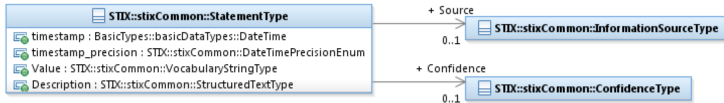
Figure 3-18. UML diagram of the StatementType class
