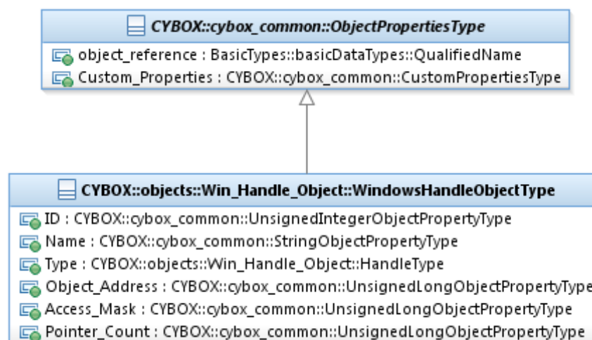
Figure 3-1. UML diagram of the WindowsHandleObjectType class
