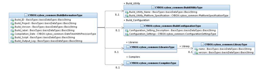
Figure 3-3. UML diagram for the BuildInformationType class
