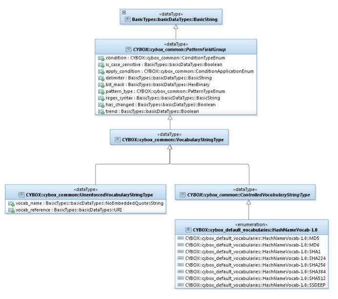
Figure 3-11. UML diagram of the CybOX Vocabulary data model
