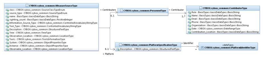
Figure 3-2. UML diagram for the MeasureSourceType class
